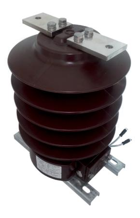
This outdoor sensor combines functions of a voltage and a current sensor in one design. Due to the structural shape and use of cycloaliphatic epoxy resin, it is adapted for outdoor application. The combined sensor is available with an insulation level up to 36 kV.
